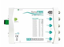
The **OPT-RX SCD MICRO** receiver converts the optical input signal into a coaxial signal available on two dCSS (SCD2) and two Legacy outputs, all with the TV signal mixed. The receiver can be powered directly from the set-top-boxes or via a dedicated DC connector. The product has a multifunctional green LED that provides the installer with various information:
